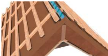
Ridge joint sealing, PAVATAPE 150
