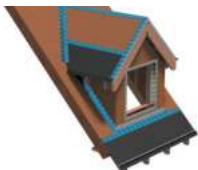
Install woodfibre insulation layers. Seal the eaves tray to the insulation, seal around the window opening and other open joints with PAVATAPE tape + primer. Taping is not necessary if ADB 'red' membrane is installed.
