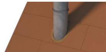
Insert the chimney with min. 50mm mineral wool or similar or as recommended by fire consultant.
