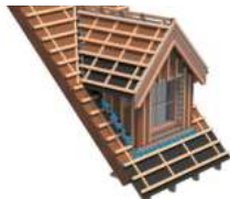
Install counter battens and tile battens. Make sure ventilation flow is not blocked.
