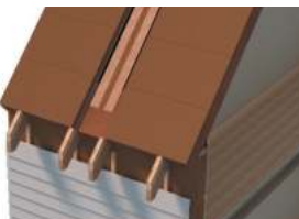
Pavatex insulation cut short at the last rafter near the party junction.
