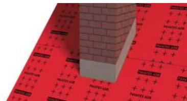
Parge the chimney to achieve a flat surface.
