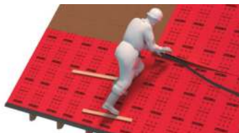
Climbing up during PAVATEX ADB breathable membrane application
