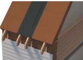
Fire rated/suitable weather membrane to cover the junctions
