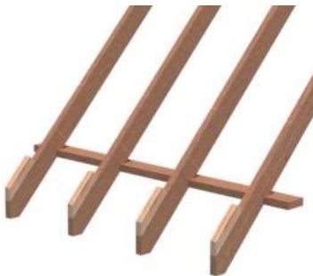
Sprocket or timber stop fixed to support the installation
