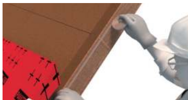
Sealing along the gable ends. PAVATAPE 12 (ADB membrane)
