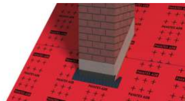
Tape the bottom edge with PAVATAPE 150. Don't forget to prime
