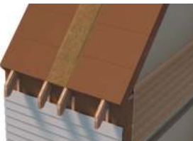
Fire rated insulation infill over the party junction.
