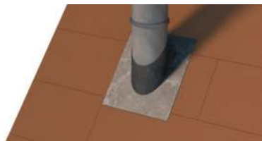
Install a fire rated chimney collar
