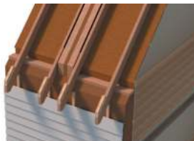
Roof party wall, timber frame
